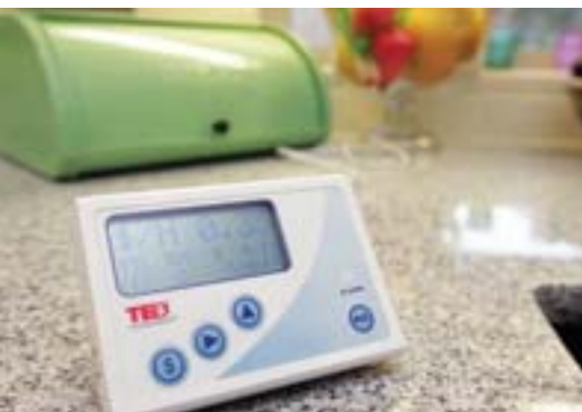
☞ One of the home's few visible signs of green technology, this monitor provides real-time, household electricity data to make homeowners aware of their actual energy usage.
